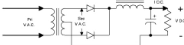
$$V_{(Peak) D.C.} = 0.45 \times \text{Sec. V.A.C.}$$
