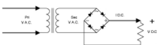
$$V_{D.C.} = 0.90 \times \text{Sec. V.A.C.}$$
