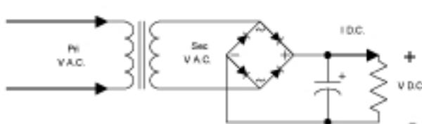
$$V_{(Peak) D.C.} = 1.41 \times \text{Sec. V.A.C.}$$
