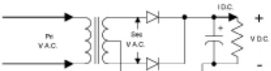
$$V_{(Peak) D.C.} = 0.71 \times \text{Sec. V.A.C.}$$
