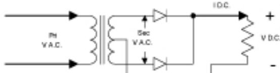
$$V_{D.C.} = 0.45 \times \text{Sec. V.A.C.}$$
