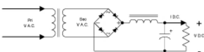
$$V_{(Peak) D.C.} = 0.90 \times \text{Sec. V.A.C.}$$
