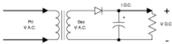
$$V_{(Peak) D.C.} = 1.41 \times \text{Sec. V.A.C.}$$
