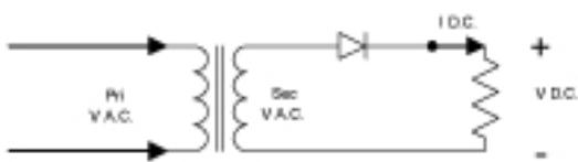
$$V_{D.C.} = 0.45 \times \text{Sec. V.A.C.}$$
